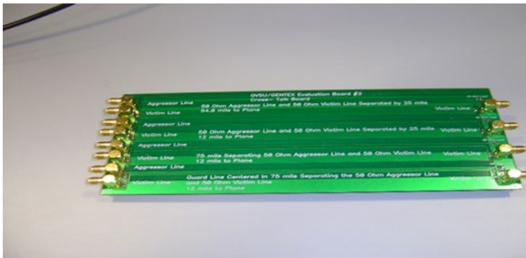
Figure 1.1 PCB used for creating crosstalk between traces.
