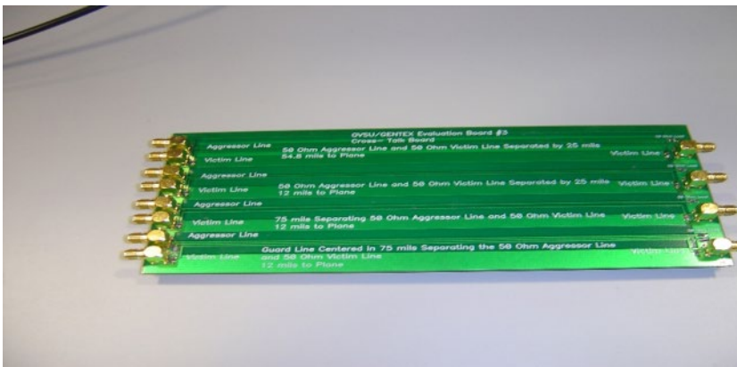
Figure 17.56 PCB used for crosstalk measurements.
