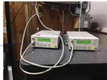
Power meters (measure forward and reverse power)
