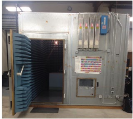
Figure A.57 Reverberation and semi-anechoic chambers for radiated immunity.
