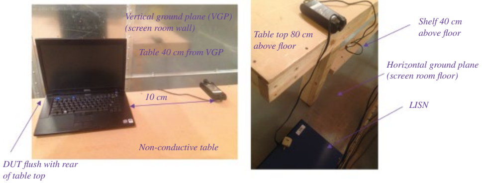
Figure A.19 DUT arrangement in a screen room for conducted emissions testing.
