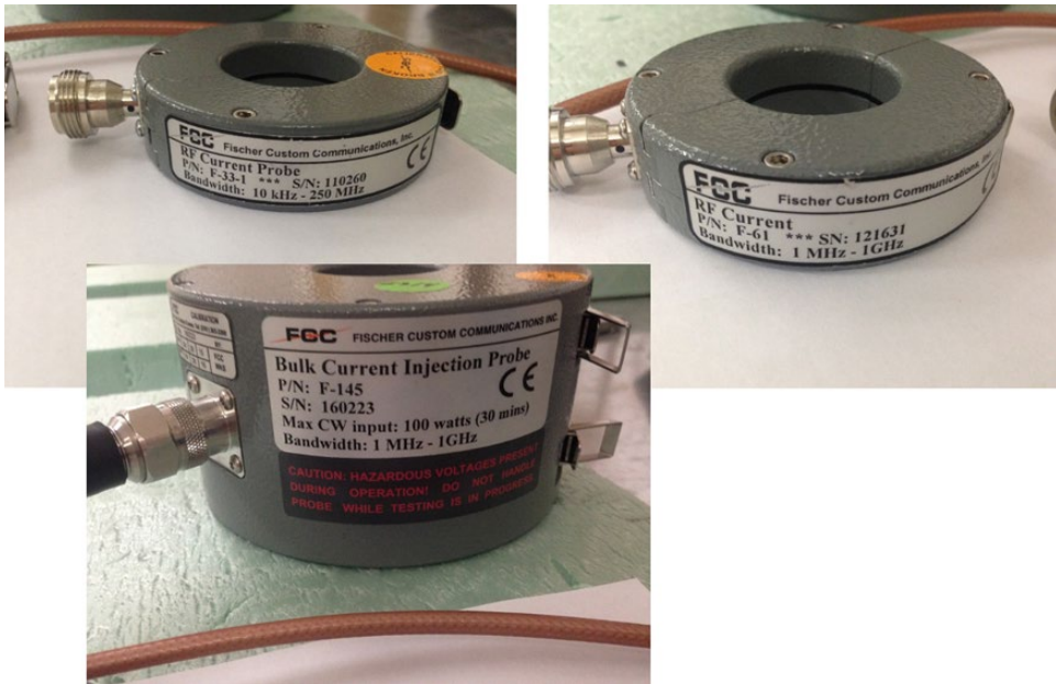
Figure 14.23 Current probes used in EMC.
