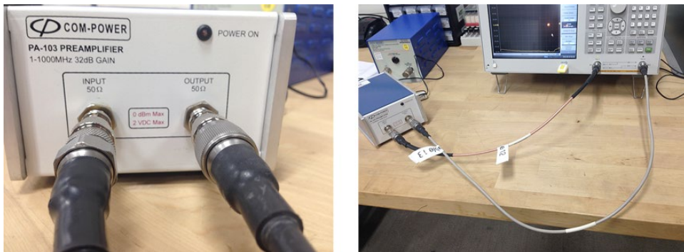
Figure 17.80 Test setup for the preamp gain measurement.
