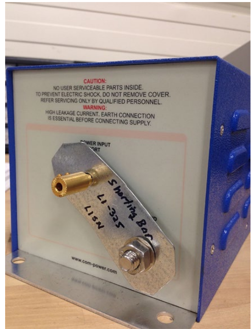
Figure 17.73 Shorting bar for impedance measurement.
