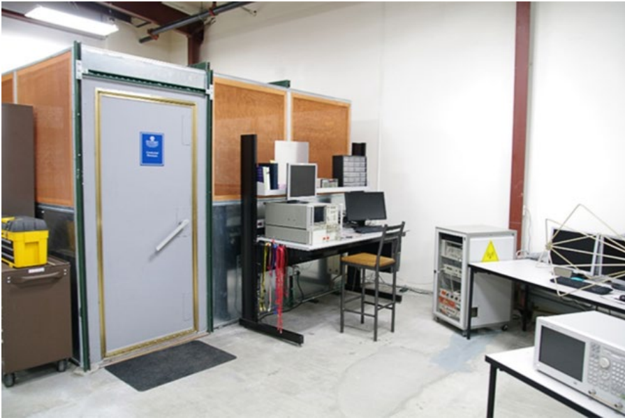
Figure A.17 Screen room for CISPR 25 conducted emissions measurements.
