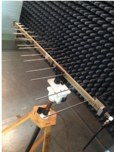
Figure A.43 Log-periodic antenna for 300–1000 MHz frequency range measurements.
