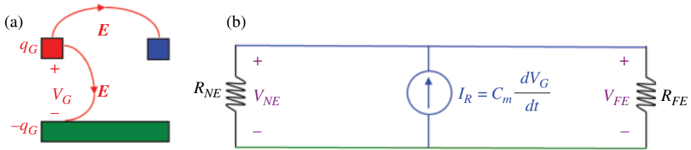
Figure 7.46 Capacitive coupling between the circuits: (a) field model, (b) circuit model.
