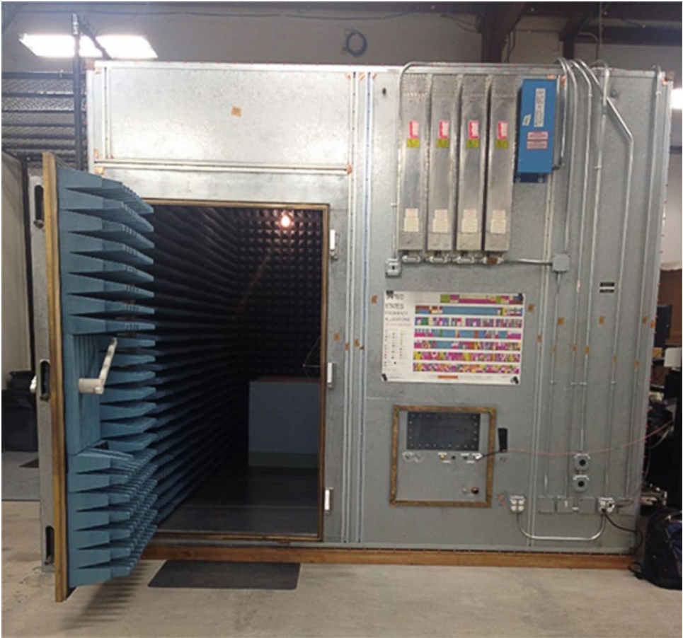
Figure A.31 A semi-anechoic chamber for radiated emissions.
