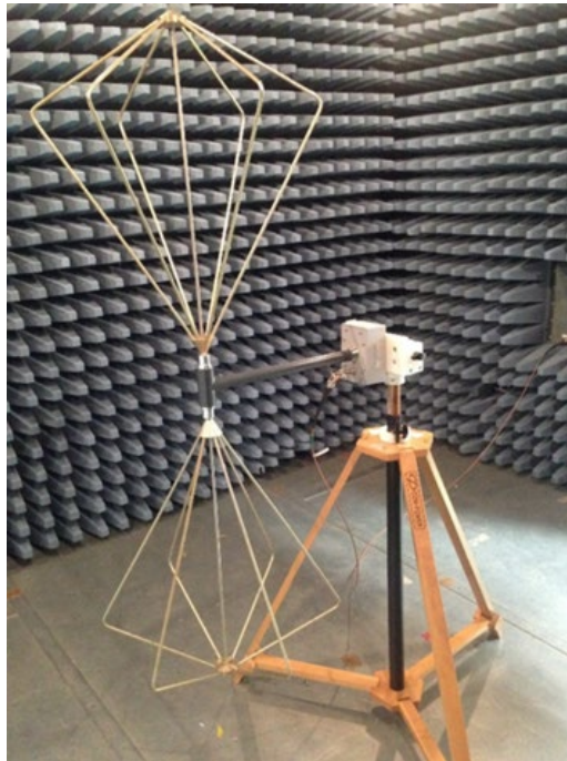
Figure A.39 Biconnical antenna for 30–300 MHz frequency range measurements.
