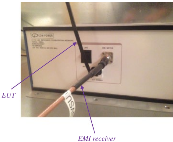
Figure A.12 FCC/CISPR22 ac LISN.
