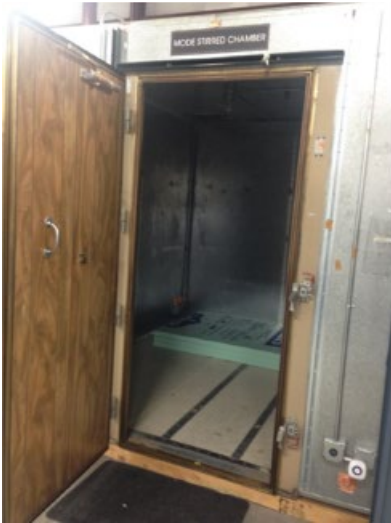
Figure A.57 Reverberation and semi-anechoic chambers for radiated immunity.
