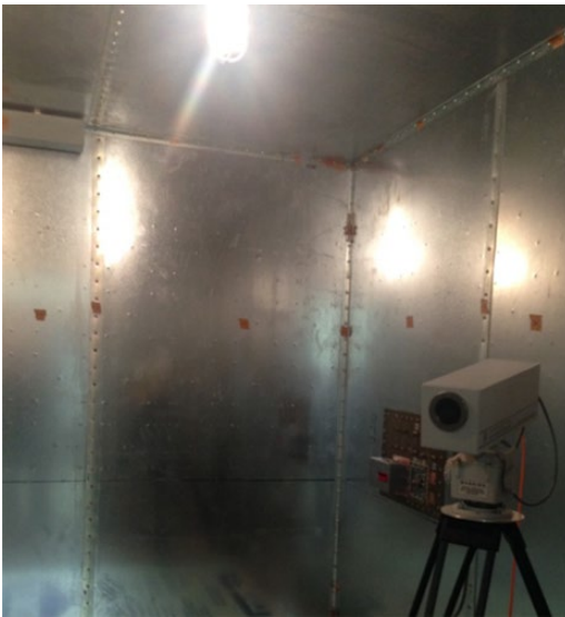
Figure A.58 Reverberation chamber is a highly reflective enclosure.
